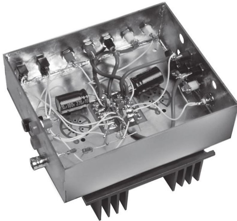
Figure 3: Inside of assembled box. Holes for components on long side were user drilled.
