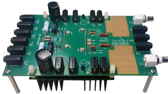
Assembled EK37 evaluation kit for MP104.
