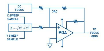
By offering multiple combinations of high speed and high voltage power amplifiers, Apex can drive the rapid correction of focus in high resolution displays. Dynamic focusing is the active correction of focusing voltage as a beam moves from the center to the edges of a CRT. Power operational amplifiers lend themselves well to this application with their ability to be connected as a summing amplifier with inputs from the nominal focus potential and the dynamic correction.
